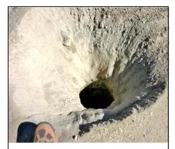
A blasting hole, about 150' deep, add 50' of explosives, fill with dirt, hook all the fuses together for a synchronized blast and stand wayyyy back.
